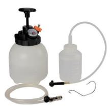
This tool is used to bleed brake or clutch hydraulics. For this purpose, the tool is connected to the hydraulic system via the compensating reservoir. The reservoir is pressurised by means of the integrated hand pump. On bleeding (on opening the bleeder nipple), the brake fluid is forced through the hydraulic pipes and replaced with an adequate amount of fresh fluid.
