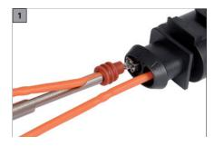
Mounting/Dismantling Tool, plastic socket bulb
