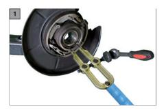
This tool is used to fit and remove circlips. Compared to conventional circlip pliers, the circlip does not need to be held under tension with physical effort. This makes installation significantly easier, even with large, heavy-duty circlips.
