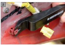
Installation Tool, charge-air hose retaining clip
