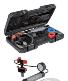
This universal tester is used to check the cooling system for leaks. It is also suitable for locating leaks on components such as cylinder head gaskets, radiators, water pumps, heater hoses and flanged connections. The special feature here is that the inflatable rubber gaiter adapts to almost every expansion tank or radiator opening, sealing them securely for reliable testing.
