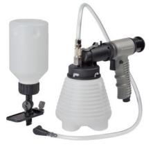
This pneumatic device is used to bleed hydraulic circuits in brake and clutch systems. The device operates according to the Venturi principle. The brake fluid is drawn off via the bleed nipple. A refiller is positioned on the expansion tank side and automatically regulates the fill level of the expansion tank.
