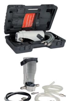
This practical hydraulic pump in a design suitable for use in workshops is used for pumping off or refilling and filling all non-easily flammable fluids, such as engine and transmission oil, radiator antifreeze, brake fluid, etc. The pump is either powered electrically, using a cordless screwdriver or alternatively also pneumatically using an air ratchet or impact wrench.
