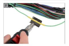
Thanks to the adjustable gas supply and the attachments included in the scope of delivery, the burner is suitable for a wide variety of operations, such as for professional heating of shrink tubing or soldering in cable lugs. with piezo ignition
