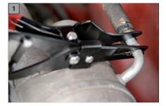
Mounting of our Herth+Buss ClipFix® spacers is sometimes difficult, depending on they ensure wide usage with the different vathe application. These pliers are designed for riants and sizes. easy mounting of Herth+Buss ClipFix®
